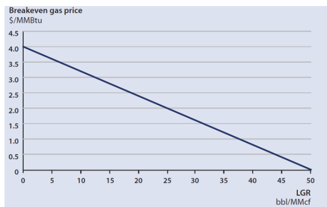
Figure 13. Impacts of liquids for breakeven prices of US shale (MIT, 2011).
