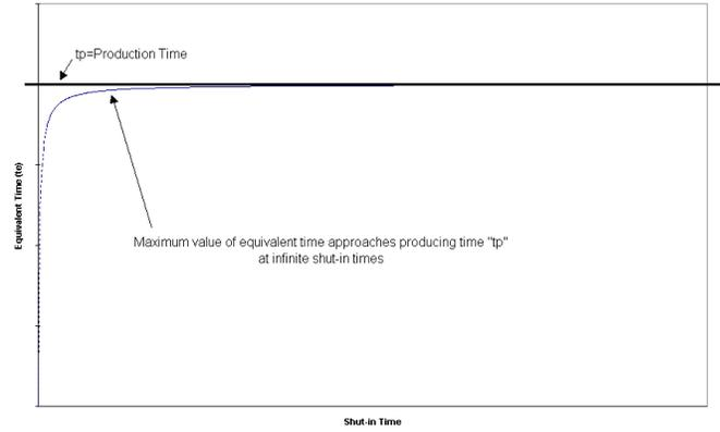
Figure 7 – Equivalent Shut-in Time as a function of Shut-in Time
