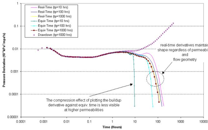
Figure 1c – Well Near One Boundary in Closed Reservoir; High Permeability (100 mD)
