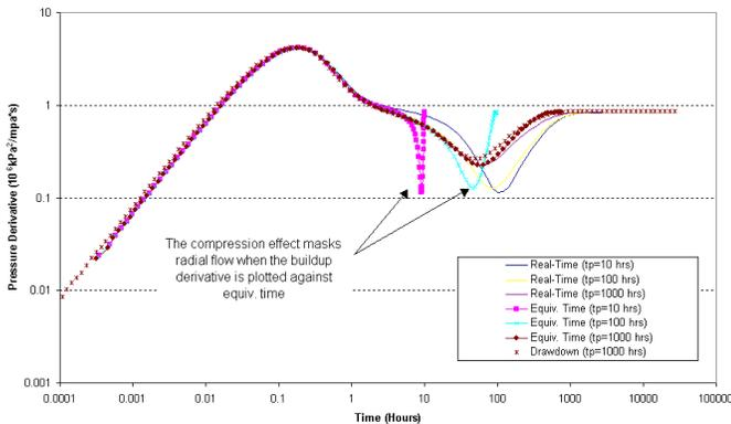
**Figure 4a – Low Interporosity Flow Coefficient (matrix permeability = 1 mD, IC = 1E-6)**
