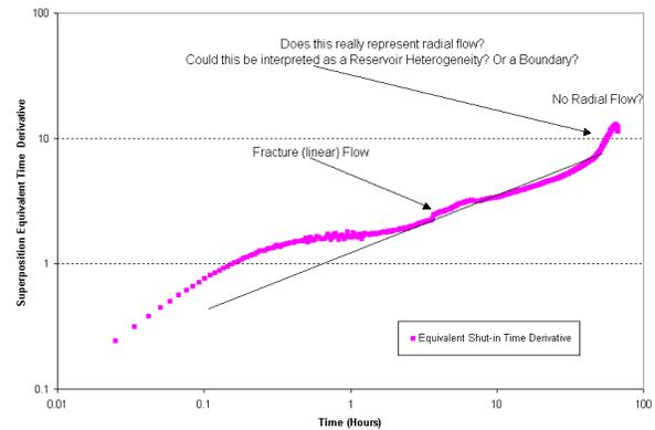
Figure 6b – Calculated Buildup Derivative (Field Example #2)
