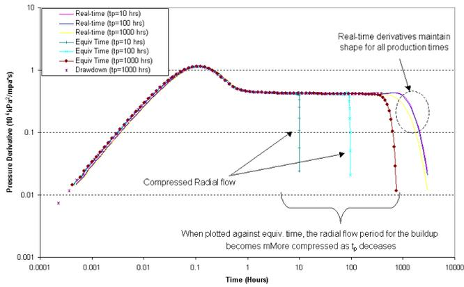
Figure 1a- Centered Well in a Closed Reservoir; Low Permeability (1 mD)
