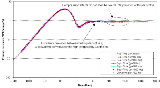
Figure 4b – High Interporosity Flow Coefficient (matrix permeability = 1 mD, IC = 1E-4)
