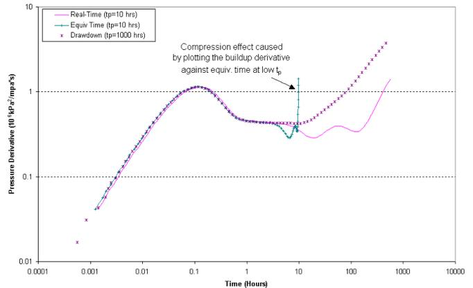
Figure 1f – Well Near Three Boundaries in a Closed Reservoir; Low Permeability (1 mD)
