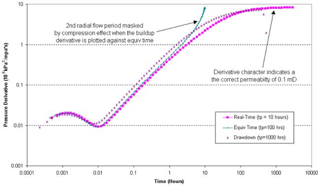
**Figure 2a- High Permeability Inner Zone (100 mD); Low Permeability Outer Zone (0.1 mD)**
