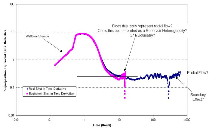
Figure 5c- Calculated Buildup Derivative (Field Example #1)
