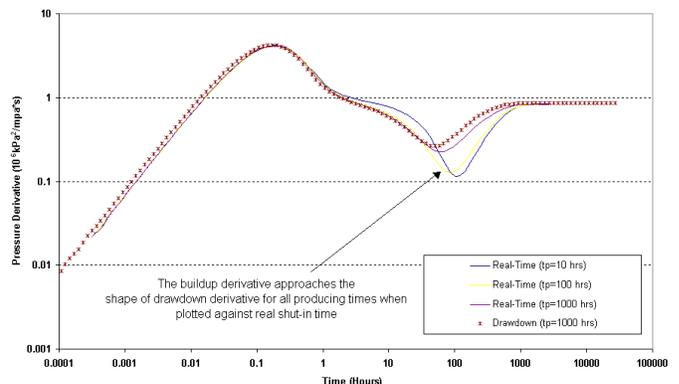
**Figure 4a.2 – Low Interporosity Flow Coefficient (matrix permeability = 1 mD; IC=1E-6)**
