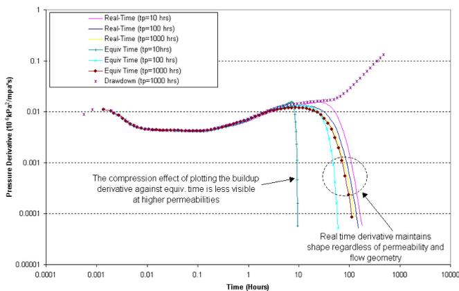
Figure 1e – Well Near Two Boundaries in a Closed Reservoir; High Permeability (100 mD)
