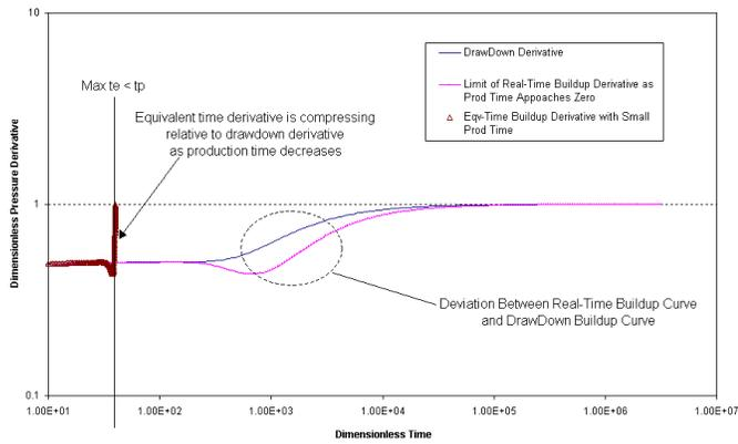
Figure 8 – Typical Derivative for a Well Near a Single No-Flow Boundary
