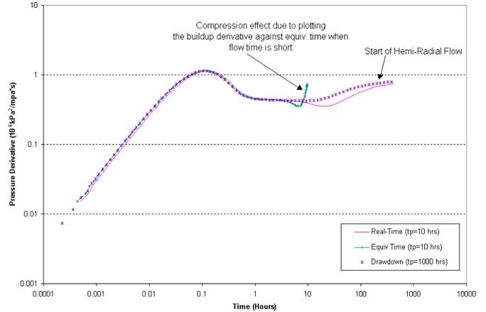
Figure 1d- Well Near One Boundary in Closed Reservoir; Low Permeability (1 mD)
