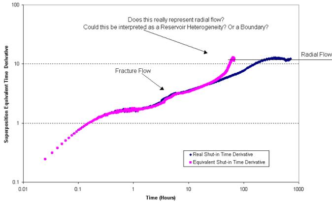
Figure 6c – Calculated Buildup Derivative (Field Example #2)
