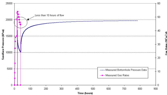
Figure 6a – Field Example #2 – Measured Rate and Pressure Data
